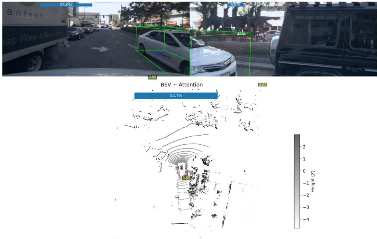
Figure 7: Raw cross-attention examples for objects (green OBB) that lie in the overlapping FOV of two cameras. In each example, a single query is used to generate the saliency maps for all camera images. Attention can be observed on the object on both overlapping images.
