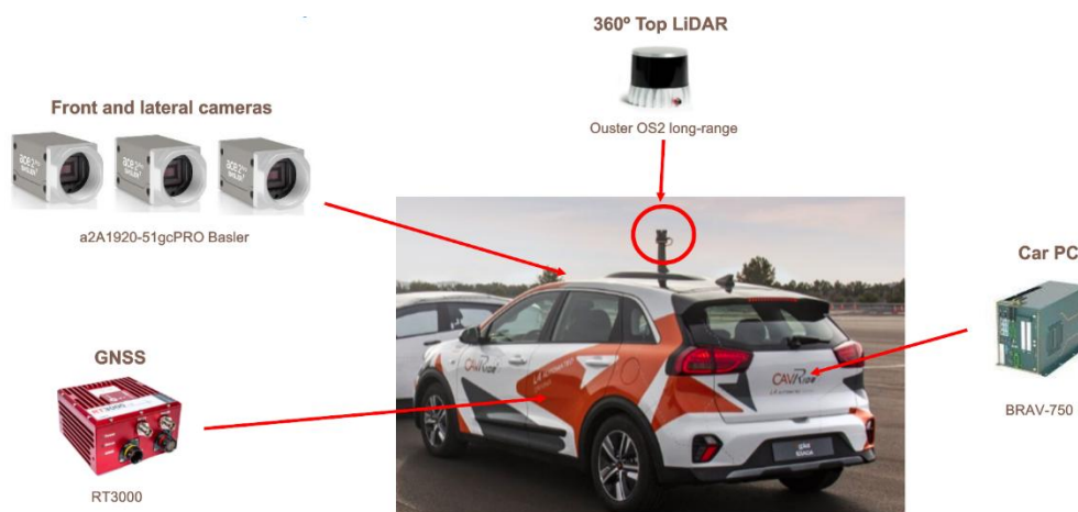
Figure 7: IDIADA's CAVride sensor setup.
