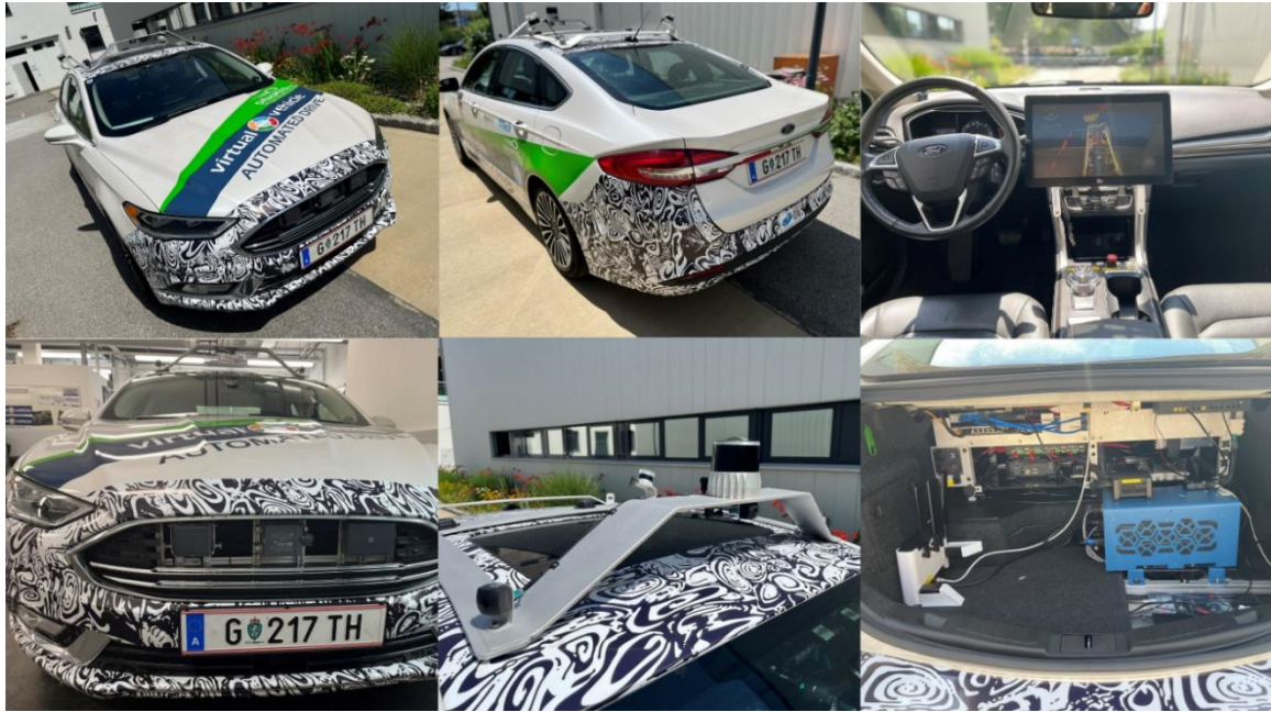
Figure 6: External and internal set-up of the demonstrator vehicle
