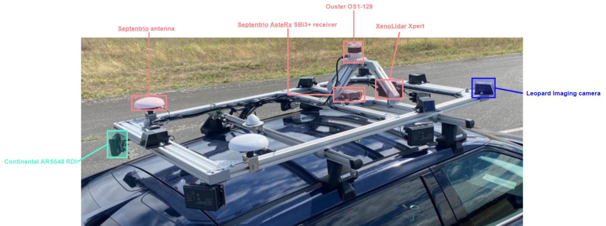
Figure 3: Perception sensors mounted in the SIE-BE roof rack
